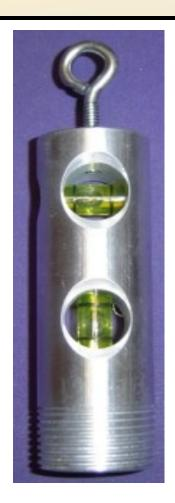
These Piping Levels were crafted by two retired UA Members. The levels have been tried and proven to be a real time saver for aligning tees, 90's, etc. Works well for welding in stubs using various nipples, bushings, or reducing couplings. With reasonable care these levels should last a Lifetime. If a thread becomes damaged, just re-tap it or run the thread over with a die.
