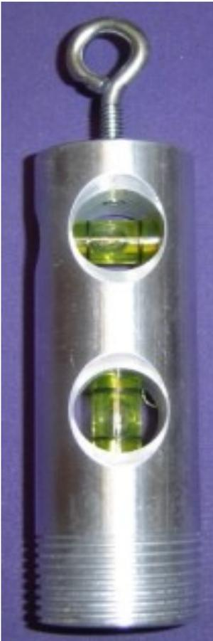
These Piping Levels were crafted by two retired UA Members. The levels have been tried and proven to be a real time saver for aligning tees, 90's, etc. Works well for welding in stubs using various nipples, bushings, or reducing couplings. With reasonable care these levels should last a Lifetime. If a thread becomes damaged, just re-tap it or run the thread over with a die.
