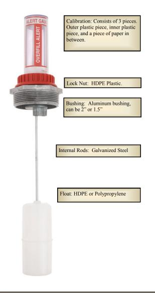
Part Number— OF-(size opening)-(overfill warning level)-(list options) Sample—OF-2-8
